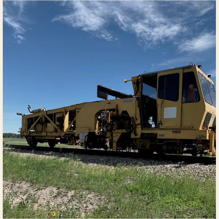
Figure 2: The Tamper at work on Wheatland Express tracks. Photo by the author
